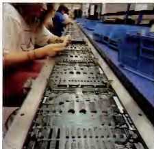
The analog and logic boards produced at Apple's Macintosh factory will pass by the stations of seven assembly workers on their way to completion.
