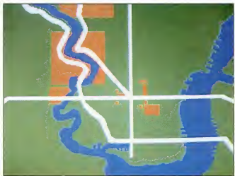
When using an optional high-resolution monitor, the Mindset computer can generate 640 \times 400 pixels of two possible colors, and in the next highest mode it displays 320 \times 200 pixels in up to 16 colors. Several graphics packages will be available under its label.
