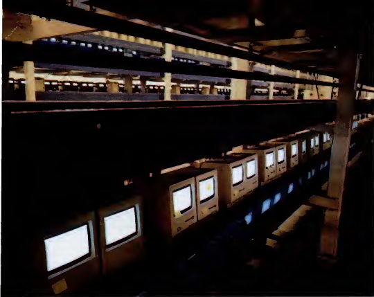
Above: Macintosh computers are tested for quality during a 24-hour burn-in cycle. Top right: A tote stacker, a crane-like vehicle used to deliver parts to workstations. Bottom right: Circuits are taken by a machine from reels and automatically inserted on printed circuit boards.
