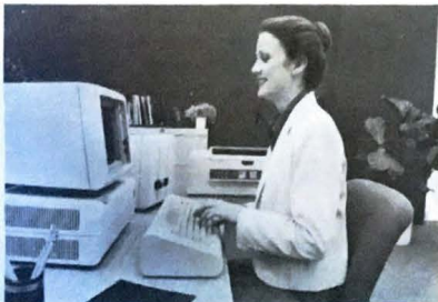
The IBM Displaywriter System consists of desk-top display and electronics modules, typewriter-like keyboard, any one of three typewriter-quality printers and removable diskette storage.
