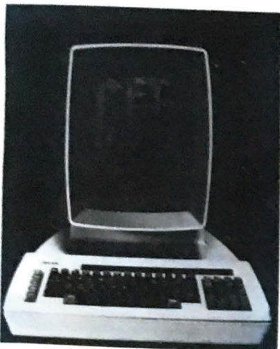
The Axix System 90 Electronic Office is a prime example of a multi-function integrated work system. It incorporates word processing, electronic mail, and administrative support functions, and fits into the traditional office environment where the principal-to-secretary relationship holds firm.
