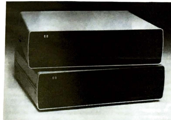
Hewlett-Packard has entered the 5.25-inch Winchester disk drive market with the 9134A (top) and the 9135A (bottom). Both models include the same 6.4-megabyte Winchester disk drive, but the 9135A also includes a 420K-byte 5.25-inch floppy disk drive. A controller, interface, and power supply are included.
